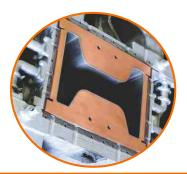
Beam Blank Mould Plate
